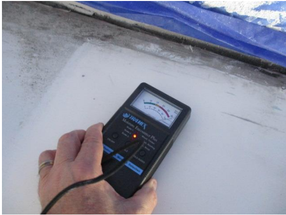
Moisture ingress due to inadequate waterproofing methods
